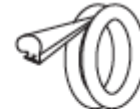
COIL DIRECTION OF 'BLUE LABEL' = QLON 9898 PT No. 02798982 (BLACK, 700m C/COIL) EUROCELL P/No 6805092R
