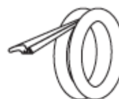
COIL DIRECTION OF STANDARD Q-LON 9821 (A) PT No. 02798210/1/2/6/8
